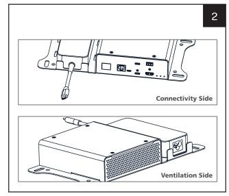
Check the orientation of the PSU. Power-In socket towards ventilation side of VXT.
