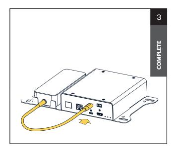
The PSU Power-Out (with USB-C connector) can now be connected to the VXT.
