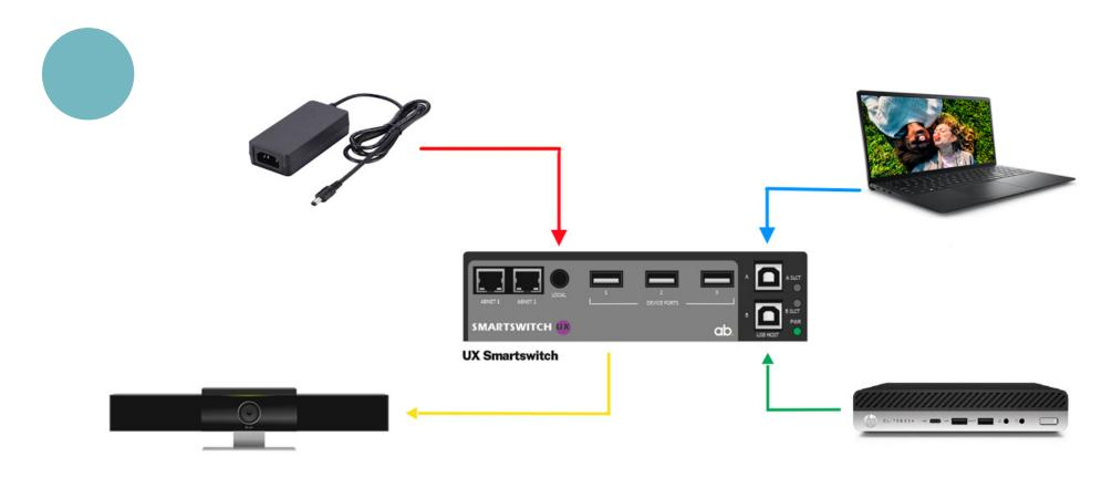
If used in Standalone mode (without a TX2 / DX2) you will require the optional power supply (part no. 900-00585) to power the UX.
