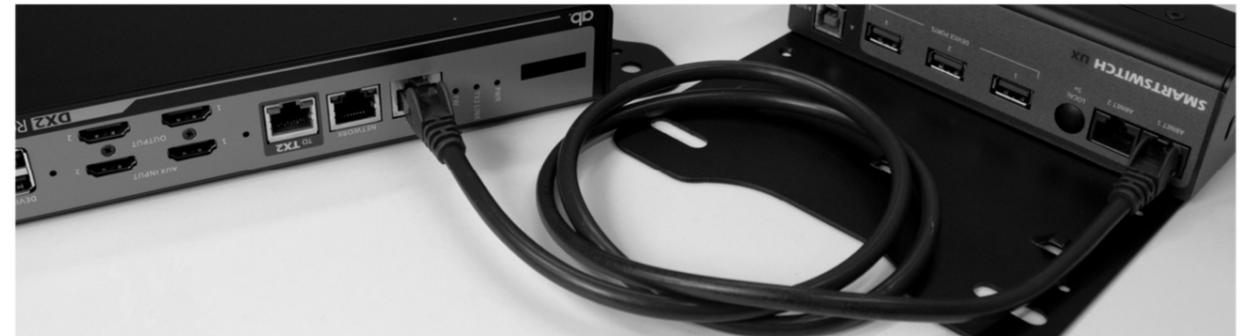
Connect the DX2 PSU, and power the system. The UX is then powered from the DX2.
