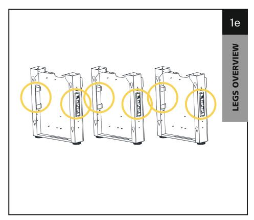
This process is applied to each of the three legs supplied ensuring that only one block per leg is fitted.
